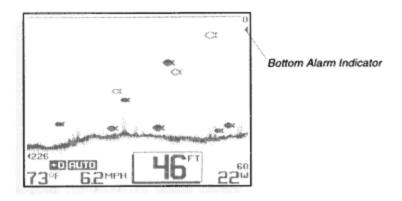
The Fish Alarm alerts you to the presence of fish, or other targets not attached to the bottom, in the water beneath your boat. The Fish Alarm has 3 different settings which correspond to the 3 different size fish targets shown on-screen.
